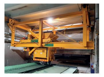
Concrete discharge and batching are carried out using eight slide gates with adjustable opening widths and a discharge roller set up in each of the buckets
