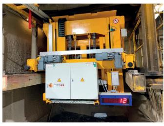
Travelling with each concrete spreader bucket are a control unit cabinet and digital weight measuring system with large screen display
