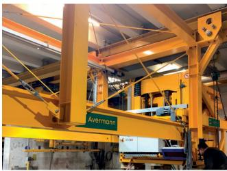
The hoisting height of each of the two concreting buckets is about 1,100 mm
